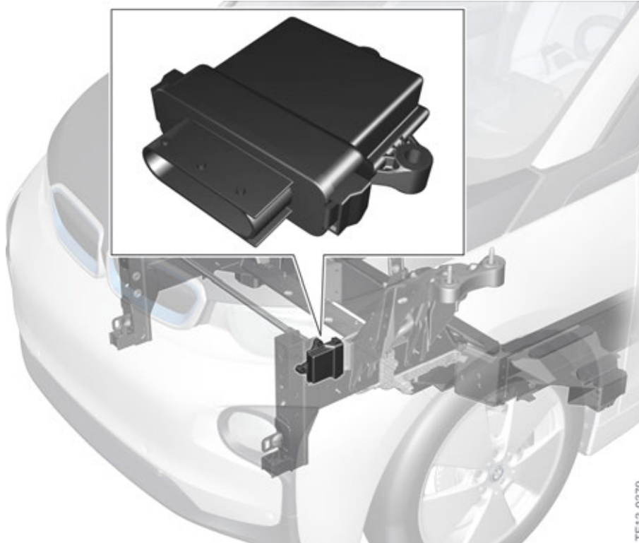
Installation location of heat pump controller, BEV only
